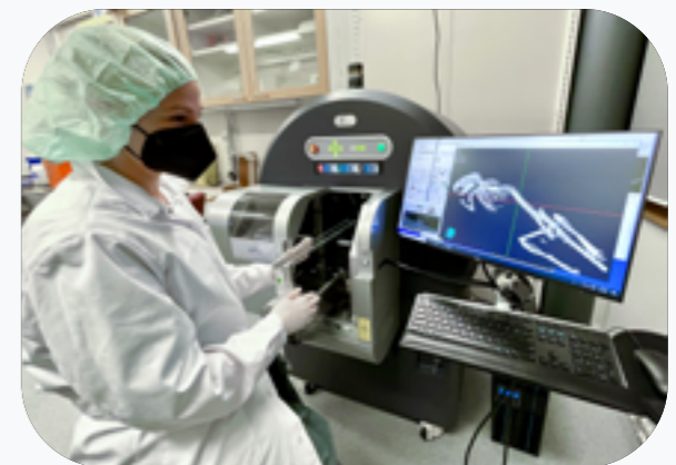
New ultra-high resolution U-CT system at the FIBI Node
