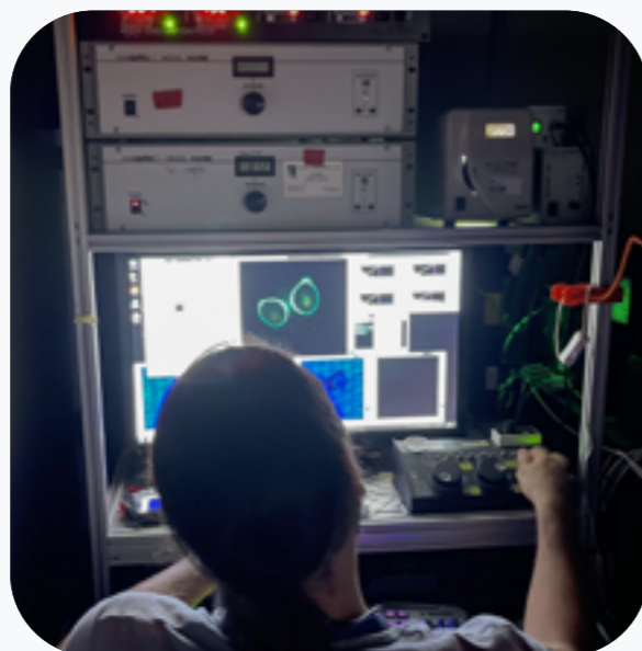
PPBI staff member acquiring images of drosophila larvae using a multi-photon microscope
