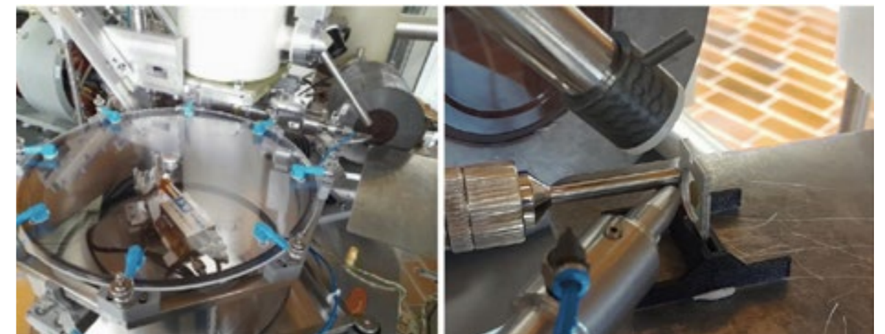
In-air PIXE developments by the imaging facility at Jožef Stefan Institute, part of our SiMBION Node. To learn more, read the paper: Isaković et al, A parallel-beam wavelength-dispersive X-ray emission spectrometer for high energy resolution in-air micro-PIXE analysis, Journal of Analytical Atomic Spectrometry , Volume 38, Issue 5, Pages 1164 - 117213 April 2023. Above image is Figure 2 from Isaković et al, 2023. https://doi.org/10.1039/D3JA00019B . CC BY-NC 3.0.
